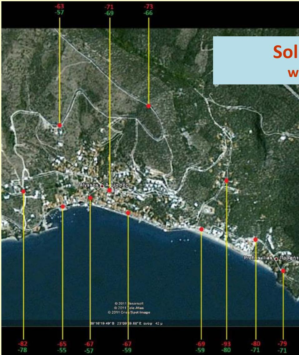
**Solution:** Replace High Gain panel antenna with high gain narrow beam VEGA antenna
